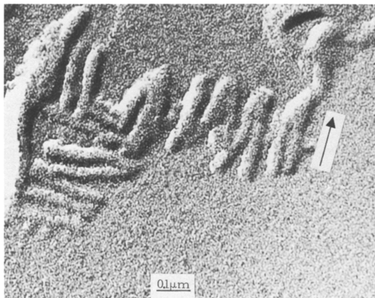
Figure 1 Electron micrograph of high molecular weight PTMT epitaxially crystallized on KCl for 5 min at 190°C. Arrow points in the substrate \langle 110 \rangle direction.
